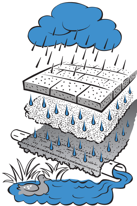
Porous paving will allow for drainage in urban areas.
